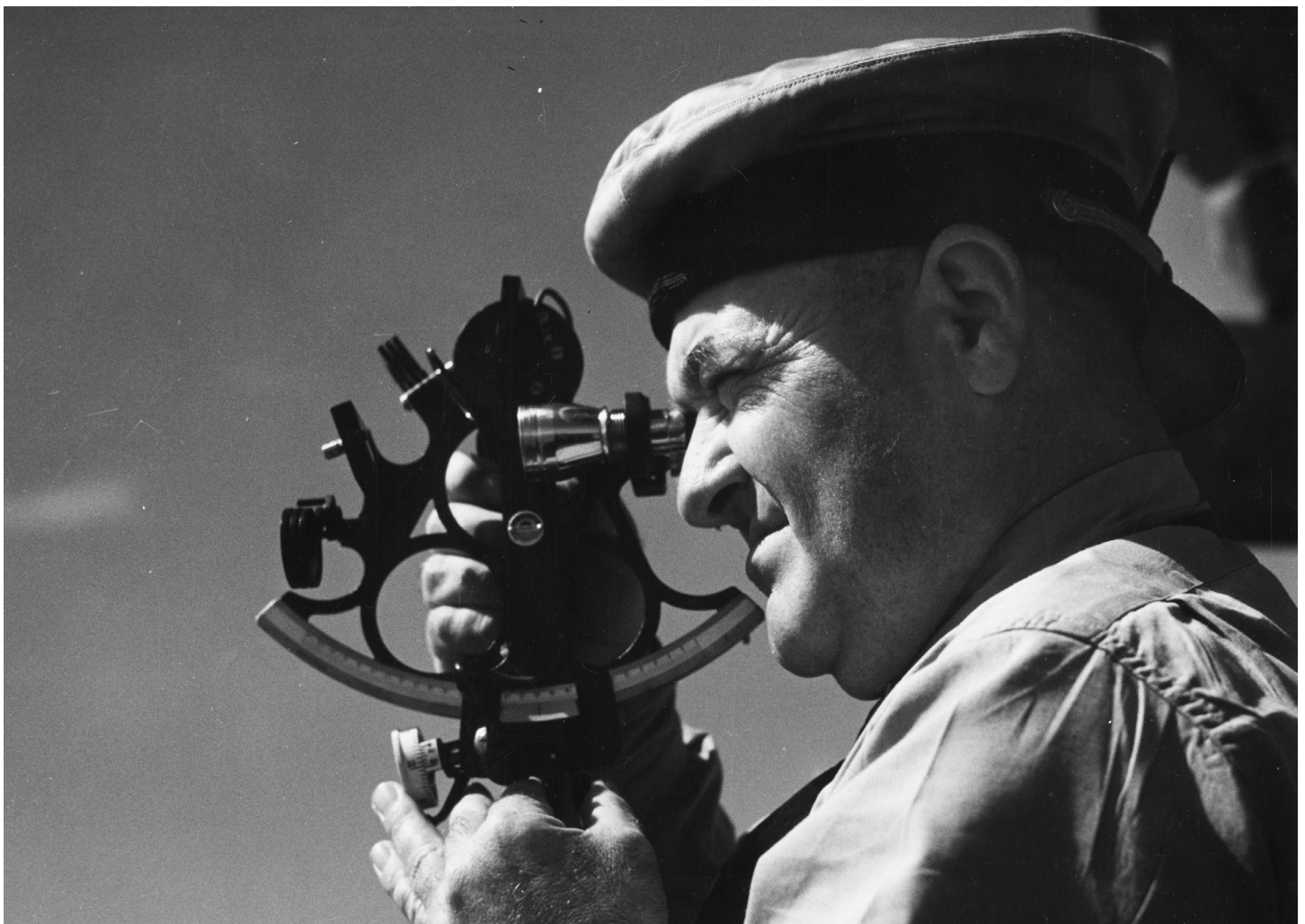
A Coast Guardsman finding his ship's position with a sextant, which uses the position of the sun to navigate. (Image: The National WWII Museum, 2015.063.091.)
